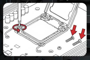
ve ILM — loosen the 4 ILM screws with the wrench and lift the ILM off; keep the motherboard screws for reuse (no screws included).
