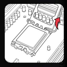
Open ILM lift the ILM lever to unlock (CPU remains in socket).
